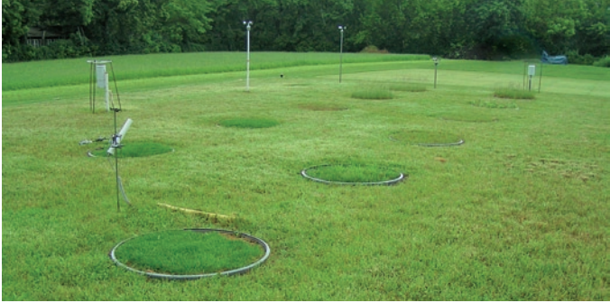
Lysimeter station at the TU Berlin in Wilmersdorf, Berlin, measuring of precipitation, infiltration and evaporation, lawn on podsol and brown earth soil types, simulated ground water levels of 1.35 and 2.10 m (s. Fig. S. 12)
