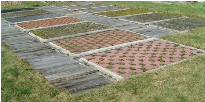
Lysimeter station at the same site for measuring the water balance of partly sealed surface reinforcements, incl. permeable asphalt, grass pavers, pre-stressed concrete pavers (s. Fig. p. 12)
