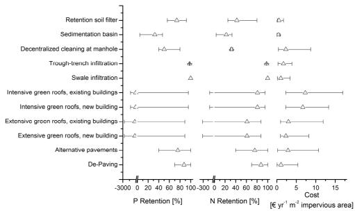
Figure 2: Average, minimal and maximal performance of selected stormwater measures regarding retention of phosphorus and nitrogen loading and present value of annual costs, including investment and operational costs and excluding land cost (adapted from Mutz et al. 2013).
